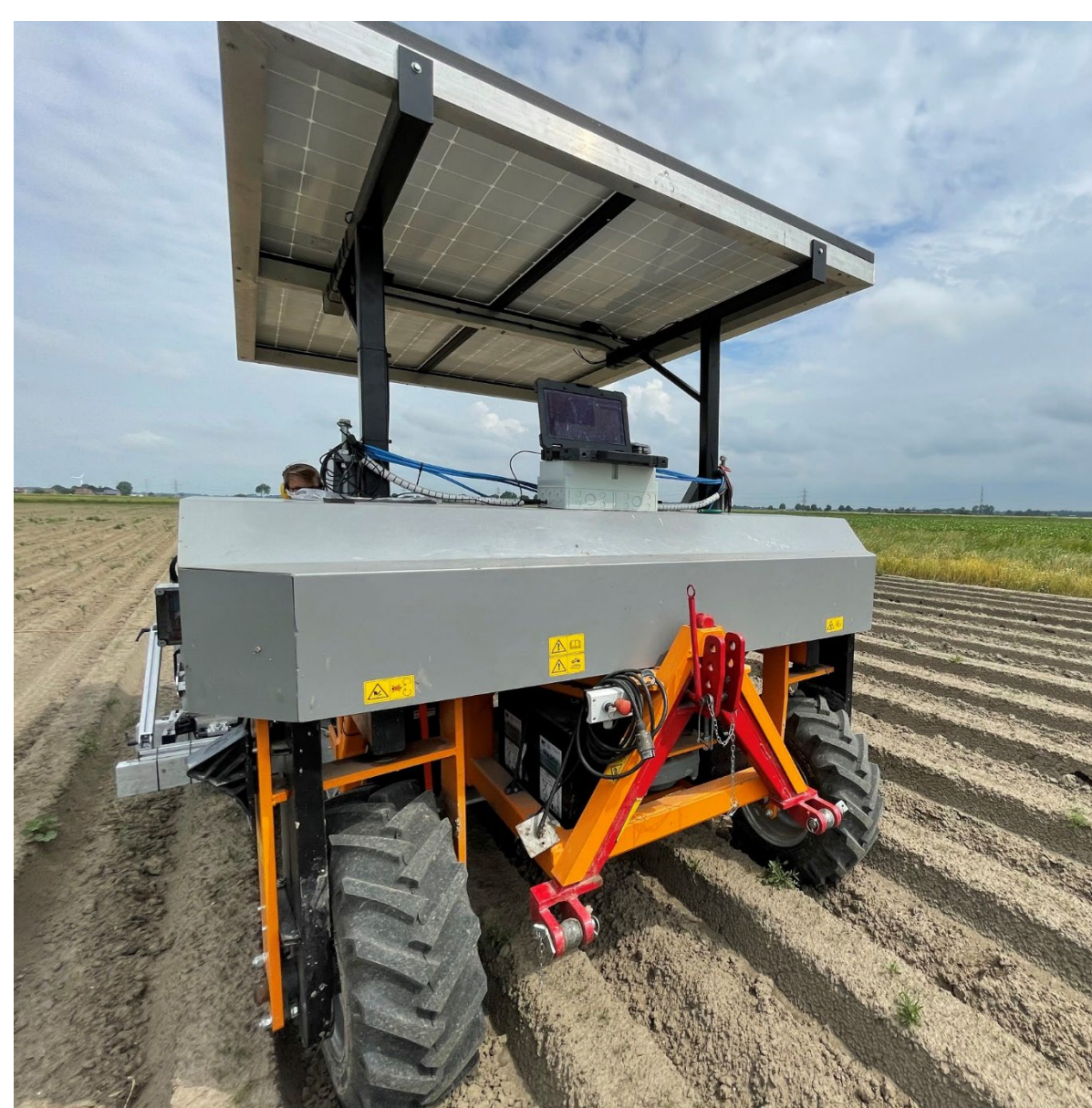
Mobile agricultural machine for automatic, herbicide-free weed control of the naiture GmbH & Co. KG, image: naiture
